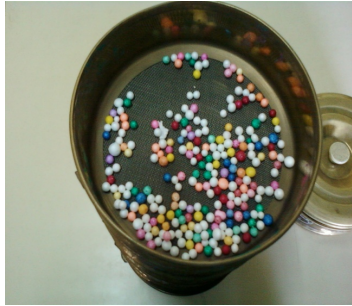
Fig. 4. (b) Sieve analysis of light weight particles
