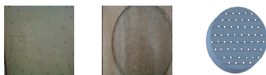
Fig. 2. (a) Triangular pitch sparger.
