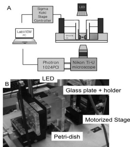
Fig. 1. (A) Schematic diagram of the dispensing system. (B) Dispensing system on inverted microscope for observation
