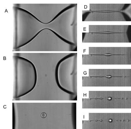
Fig. 2. (A)-(C) Satellite formation in 6 cSt silicone oil. time step between (A) and (B) is 1/1000 s. (D)-(I) Thread necking and collapsing in 100 cSt silicone oil. time step between images is 1/2250 s.
