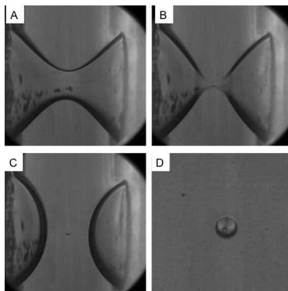
Fig. 4. Single encapsulation of 11  $\mu\text{m}$  polystyrene microparticle.
