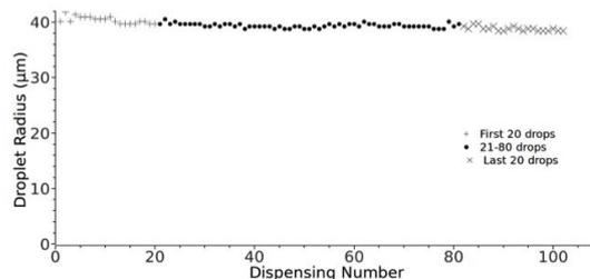
Fig. 3. Droplet size during 100-drop-dispensing out of a single 1  $\mu\text{L}$  droplet.
