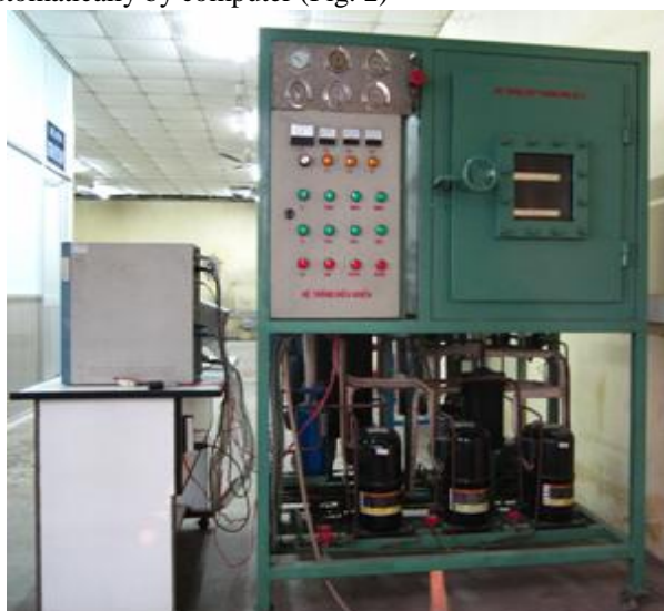
Fig. 2. The freeze drying system DS-3 with the auto-freezing (-50÷-45)°C
