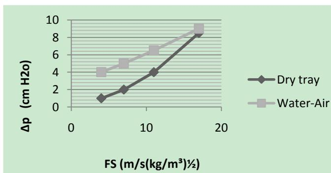
Fig. 5. Pressure drop for the centrifugal tray
