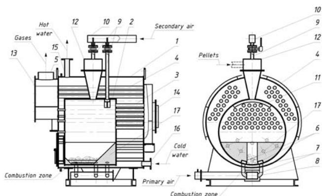
Fig. 2. Experimental boiler (hot model) diagram
