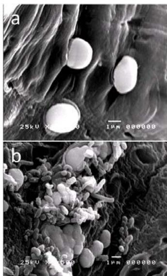
Fig. 4. SEM images of the microbial cells at 7,500× (a) before use, (b) after use for 10 cycles.
