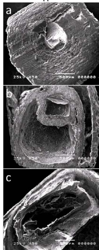
Fig. 3. SEM images of the cross-sectional BA-entrapped cells at 50 $\times$  (a) before use, (b) after use for 10 cycles, and (c) after use for 30 cycles.
