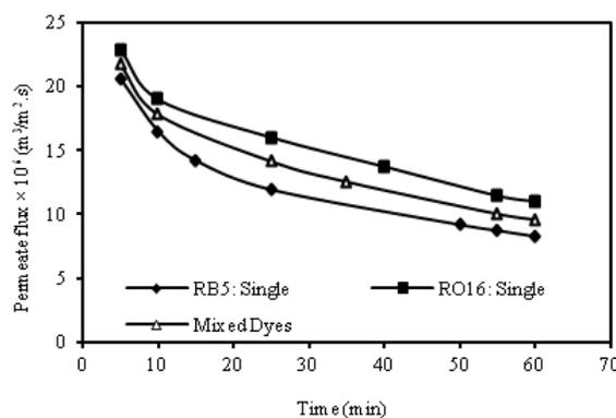
Fig. 8. Variation of permeate flux with time for MEUF of single dye and mixed dyes for RB5 and RO16
