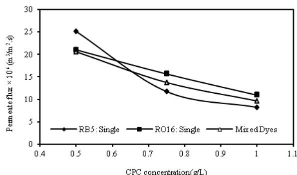
Fig. 9. Permeate flux for MEUF of single dye and dyes mixture for RB5 and RO16 after 1 hour of experiment at CPC concentration range between 0.5 g/L to 1.0 g/L
