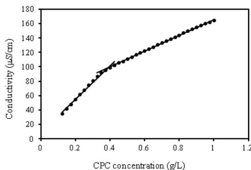
Fig. 5. Critical micelle concentration of CPC via conductivity method.
