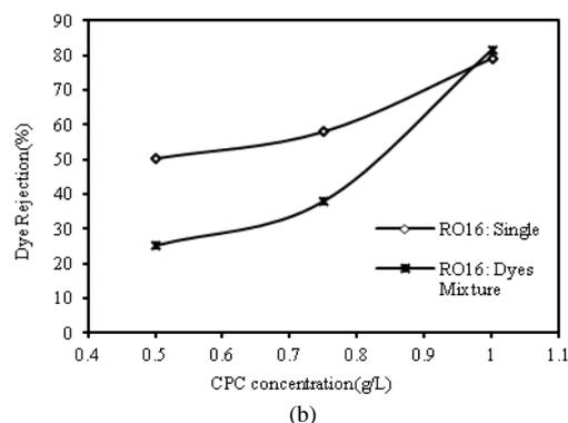
Fig. 7. Dyes rejection (RB5 and RO16) for MEUF of single dye and dyes mixture after 1 hour of experiments at CPC concentration range between 0.5 g/L to 1.0 g/L.
