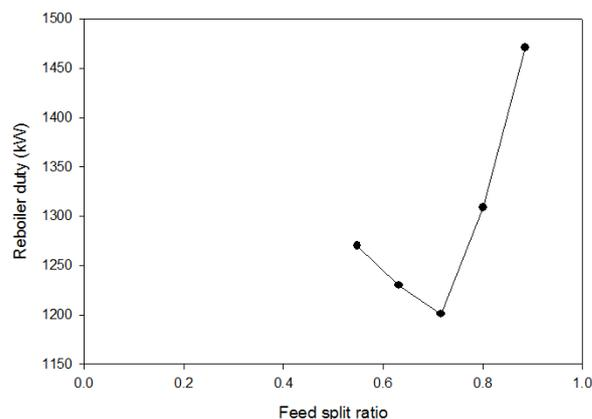
Fig. 3. Effect of feed split ratio on the reboiler duty.
