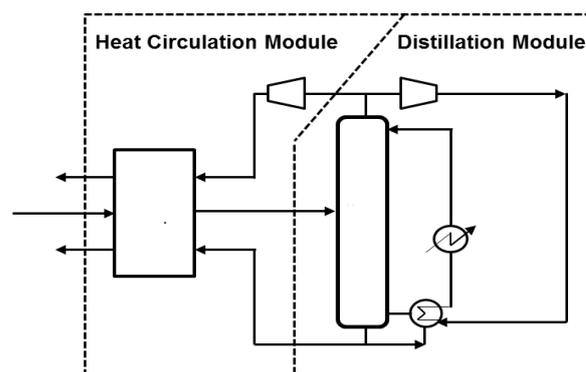
Fig. 1. Self-heat recuperative distillation process.
