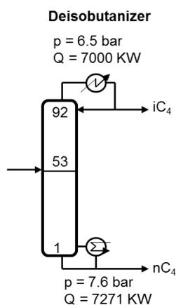
Fig. 2. Simplified flow sheet illustrating the conventional column – deisobutanizer.
