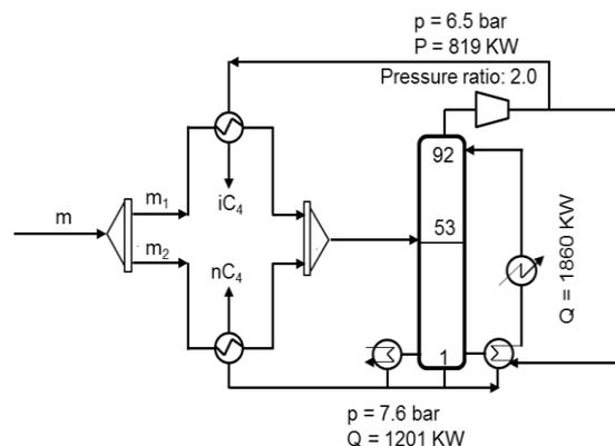
Fig. 4. Simplified flow sheet illustrating the self-heat recuperative distillation process.
