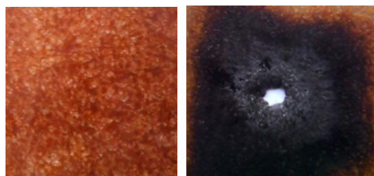
Fig. 1. Specimen before and after tested of phenolic resin/fiber glass
