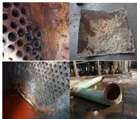
Fig. 1. Corrosion of the equipments during vanadium production
