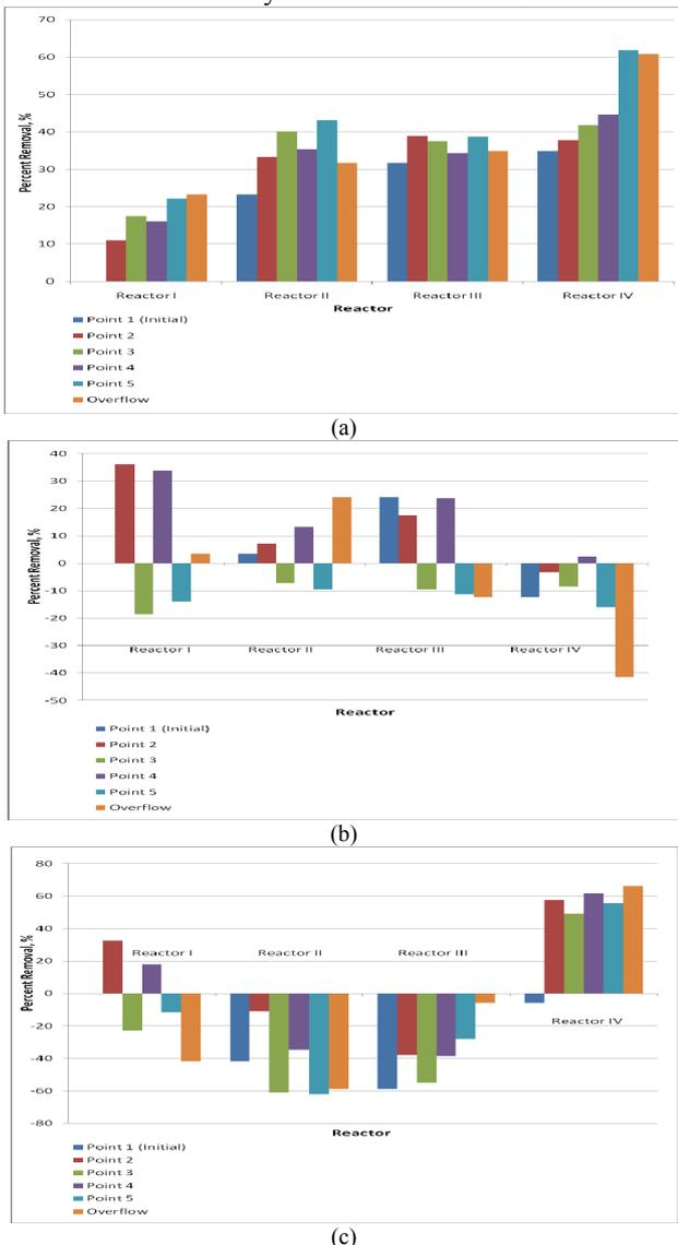
Fig. 4. Percentage removal of (a) AN, (b)  $\text{TNO}_x\text{-N}$  and (c)  $\text{NO}_2\text{-N}$  for Reactor I, II, III and IV at different sampling point.
