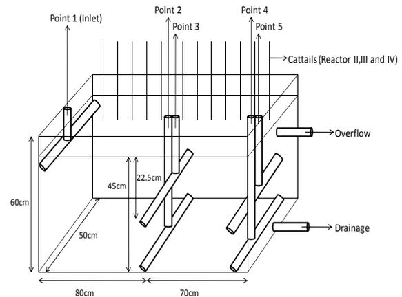
Fig. 1. Schematic diagram of reactor.
