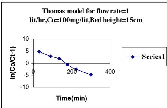
For the above fig. we can draw the straight line passing through max. points we get following Straight line equation  $y = -0.036x + 8$
