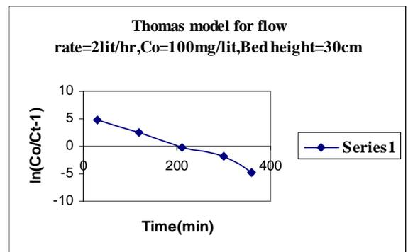
For the above fig. we can draw the straight line passing through max. points we get following Straight line equation  $y = -0.023x+6$
