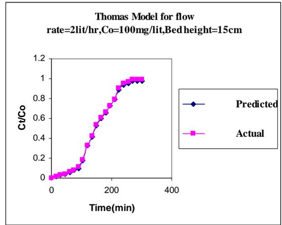
Fig-4.7 Thomas Model for Flow rate 2Lit/hr, Co=100mg/lit, Bed height=15cm
