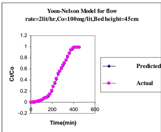
Fig-4.15 Yoon-Nelson Model for Flow rate 2Lit/hr, Co=100mg/lit, Bed height=45cm
