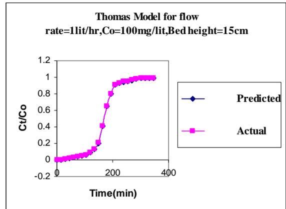
Fig-4.4 Thomas Model for Flow rate 1Lit/hr, Co=100mg/lit, Bed height=15cm
