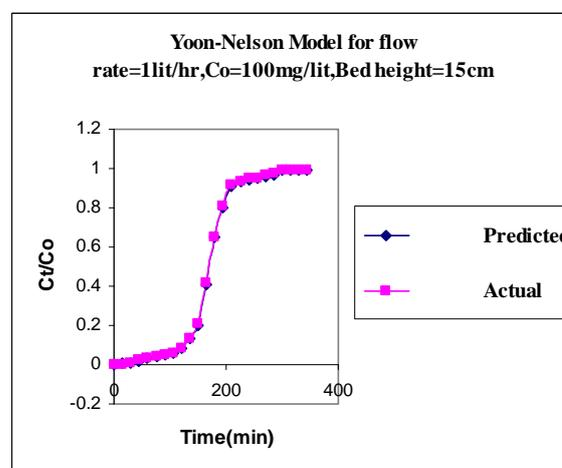
Fig-4.10 Yoon-Nelson Model for Flow rate 1Lit/hr, Co=100mg/lit, Bed height=15cm
