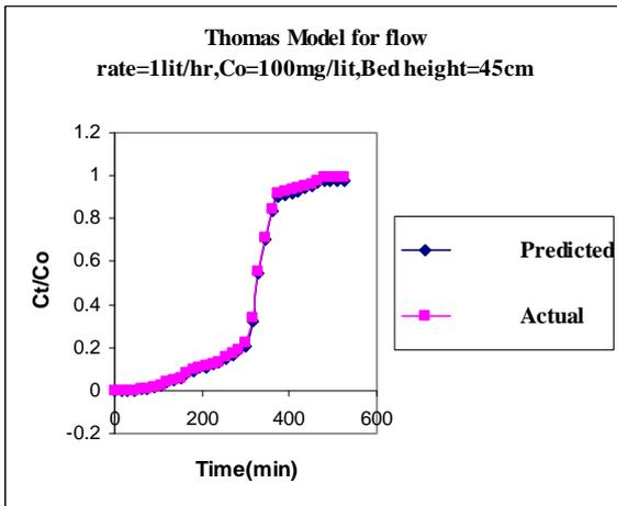
Fig-4.6 Thomas Model for Flow rate 1Lit/hr, Co=100mg/lit, Bed height=45cm
