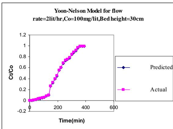
Fig-4.14 Yoon-Nelson Model for Flow rate 2Lit/hr, Co=100mg/lit, Bed height=30cm
