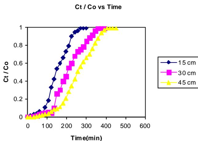
Fig. 4.2 Effect of bed height with respect to time on removal of Acid orange– II by BFA (  $C_0 = 100$  mg/lit, flow rate = 2.0 lit/hr)
