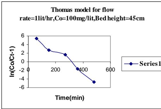
For the above fig. we can draw the straight line passing through max. points we get following Straight line equation  $y = -0.023x+7$
