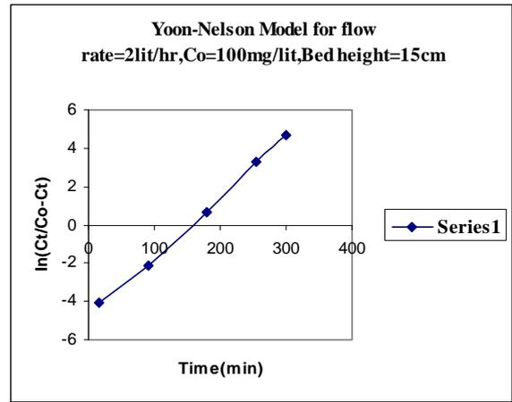
For the above fig. we can draw the straight line passing through max. points we get following Straight line equation  $y = 0.03x - 5$
