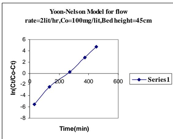
For the above fig. we can draw the straight line passing through max. points we get following Straight line equation  $y = 0.024x - 8.2$
