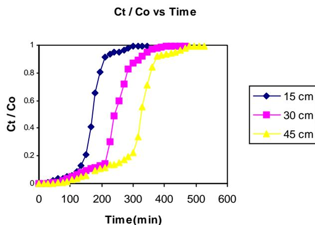
Fig. 4.1 Effect of bed height with respect to time on removal of Acid orange – II by BFA (  $C_0 = 100$  mg/lit, flow rate = 1.0 lit/hr)
