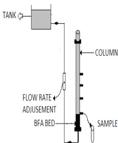
Fig. 2.1 Experimental set-up of adsorption Column
