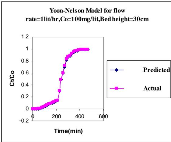
Fig-4.11 Yoon-Nelson Model for Flow rate 1Lit/hr, Co=100mg/lit, Bed height=30cm
