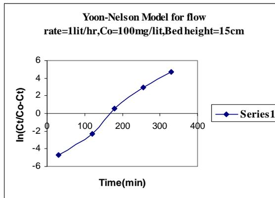
For the above fig. we can draw the straight line passing through max.points we get following Straight line equation  $y = 0.03x - 8$
