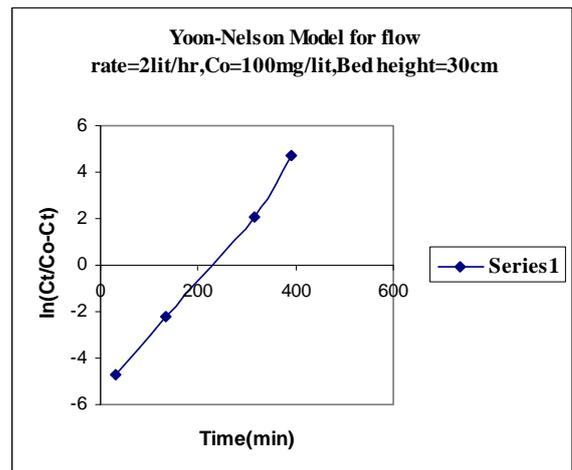
For the above fig. we can draw the straight line passing through max. points we get following Straight line equation  $y = 0.026x - 6$
