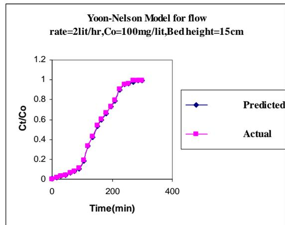
Fig-4.13 Yoon-Nelson Model for Flow rate 2Lit/hr, Co=100mg/lit, Bed height=15cm
