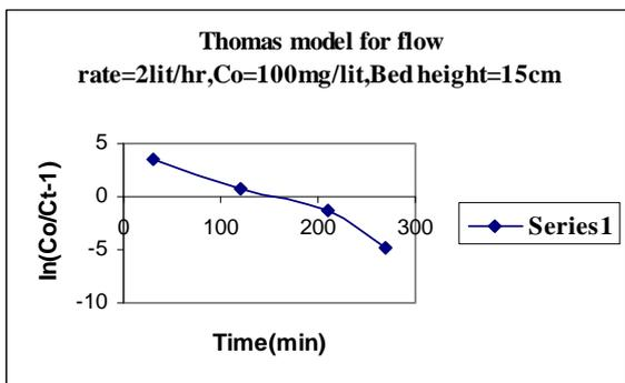
For the above fig. we can draw the straight line passing through max. points we get following Straight line equation  $y = -0.034x+6$
