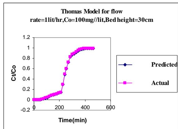
Fig-4.5 Thomas Model for Flow rate 1Lit/hr, Co=100mg/lit, Bed height=30cm
