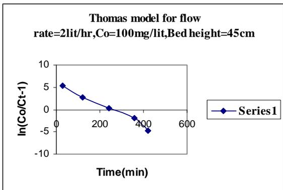
For the above fig. we can draw the straight line passing through max.points we get following Straight line equation  $y = -0.022x + 7$
