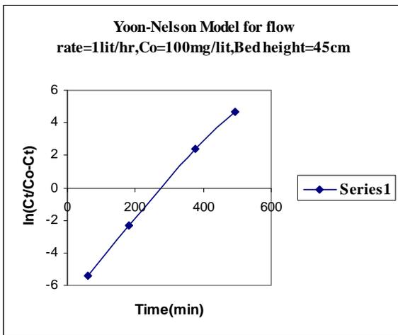
For the above fig. we can draw the straight line passing through max. points we get following Straight line equation  $y = 0.023x - 10$
