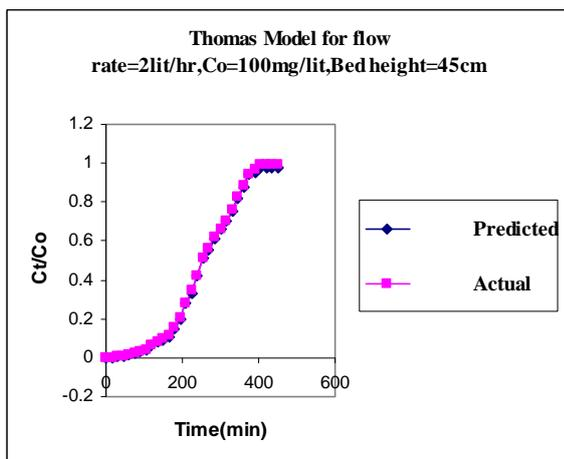
Fig-4.9 Thomas Model for Flow rate 2Lit/hr, Co=100mg/lit, Bed height=45cm
