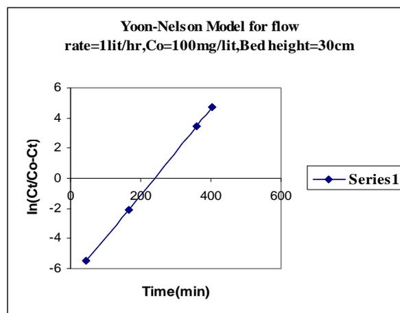
For the above fig. we can draw the straight line passing through max.points we get following Straight line equation  $y = 0.028x - 12$
