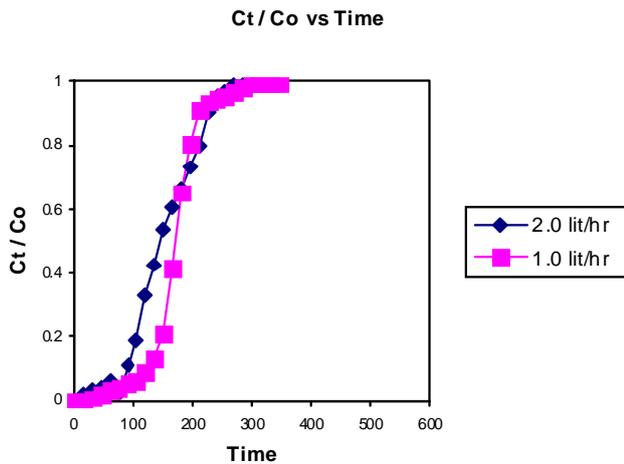
Fig. 4.3 Effect of flow rate with respect to time on removal of Acid orange- II by BFA (  $C_0 = 100$  mg/lit, bed height =15 cm)
