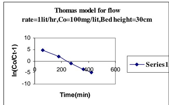
For the above fig. we can draw the straight line passing through max. points we get following Straight line equation  $y = -0.027x + 6$
