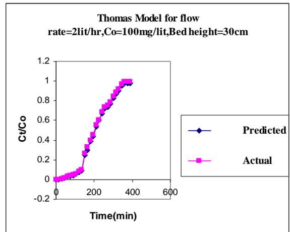
Fig-4.8 Thomas Model for Flow rate 2Lit/hr, Co=100mg/lit, Bed height=30cm
