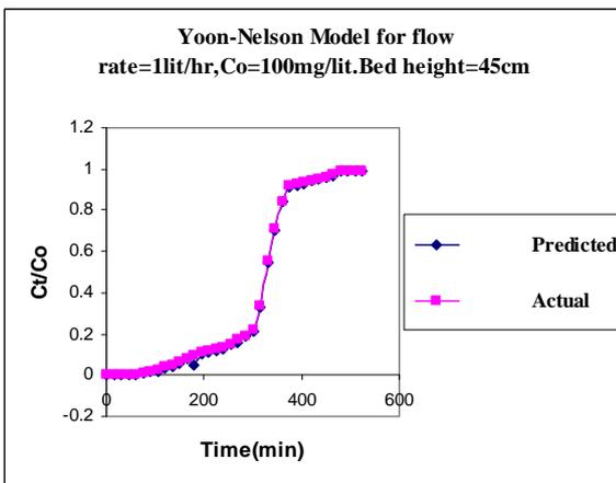
Fig-4.12 Yoon-Nelson Model for Flow rate 1Lit/hr, Co=100mg/lit, Bed height=45cm
