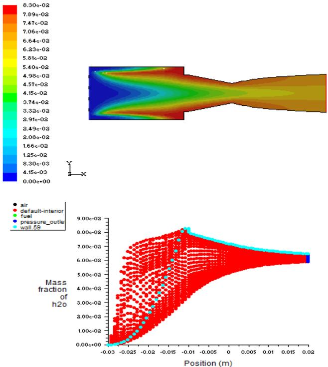
Figure-8 Mass fraction of H<sub>2</sub>O
