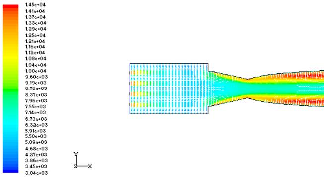
Figure- 4 Turbulence Intensity
