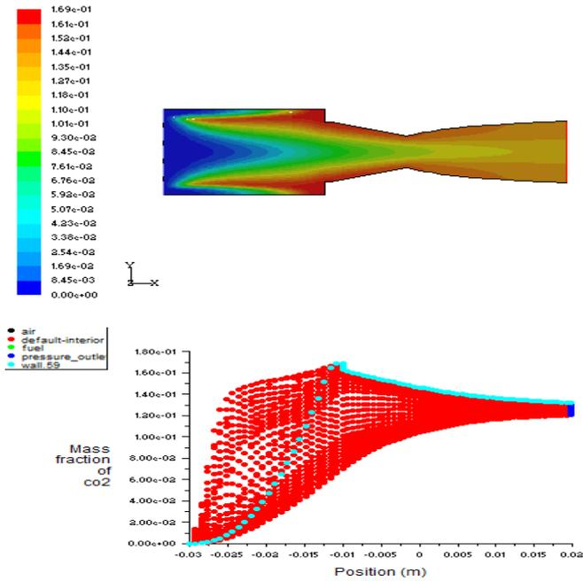
Figure-7 Mass fraction of CO<sub>2</sub>
