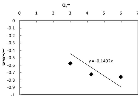
Figure 5. Graph of  $\ln(S_e/S_i)$  versus  $Q_v^{-0.5}$  for treatability constant determination
