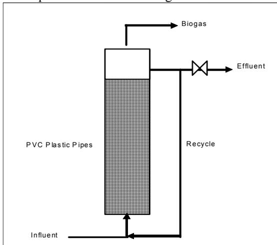
Figure 2. Schematic diagram of an Anaerobic Fixed Film Reactor
