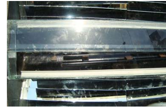
Fig 5. Solar distiller with Steel billets.
