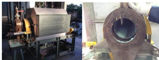
Fig. 2. Photographs of the rotary kiln used in the experiment.
