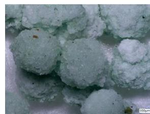
Fig. 5. Photograph of the dust fused with NaOH (1:1) using the rotary kiln.
