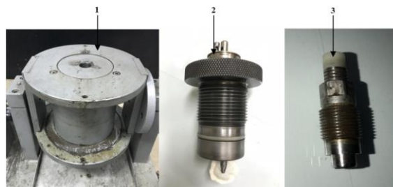
1-CV; 2-Firing block with igniter bag; 3-Pressure transducer Fig. 2. CV system.
