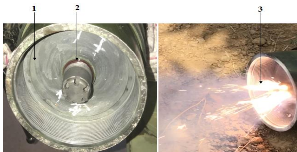
1-Dummy shell base; 2-Igniter assembly; 3-Igniter flame Fig. 9. Igniter firing.
