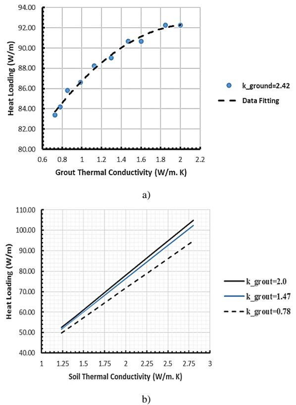
Fig. 5. a) Heat loading variation with grout thermal conductivity; b) Heat loading variation with soil thermal conductivity.
