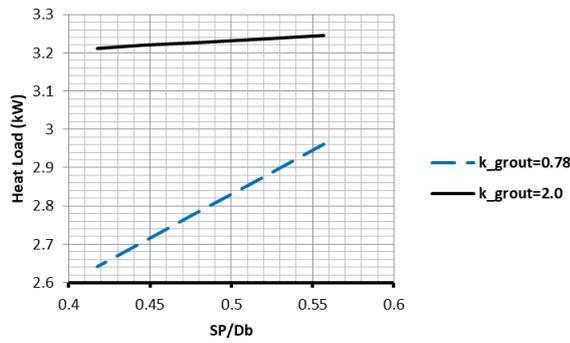
Fig. 6. Borehole heat load variation with configuration factor at soil thermal conductivity of (2.42) W/m.K.
