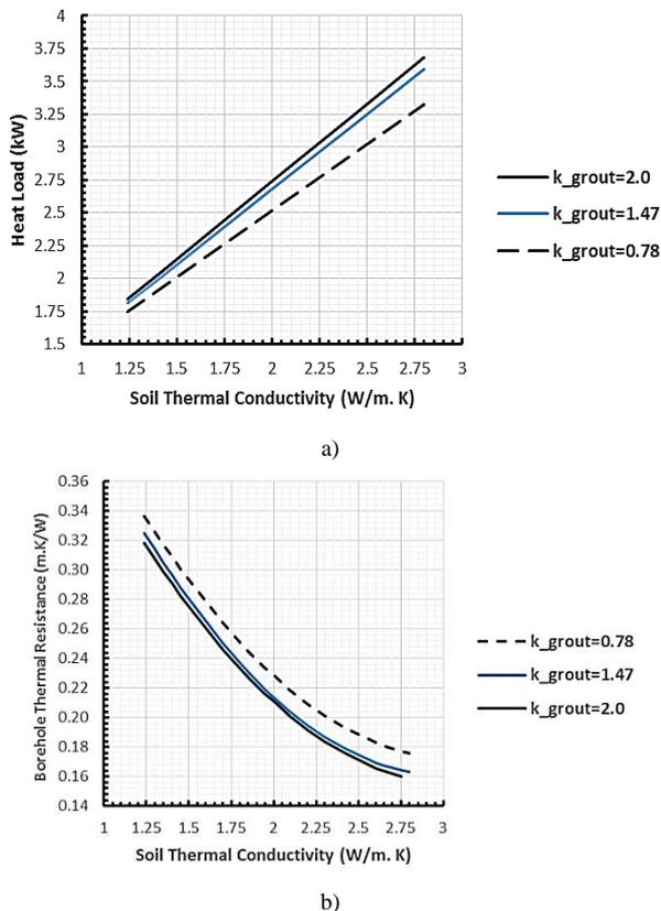
Fig. 4. a) Heat load variation with soil thermal conductivity; b) Total borehole thermal resistance variation with soil thermal conductivity.
