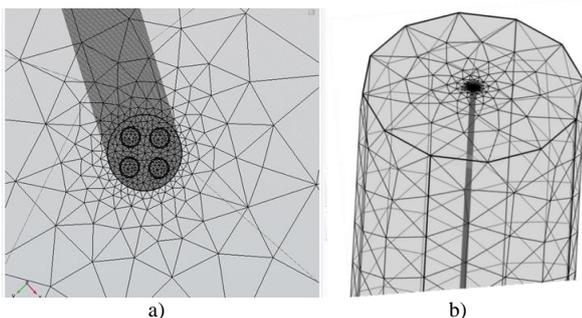
Fig. 2. a) The generated mesh of the borehole geometry; b) A general view for the model mesh generation.
