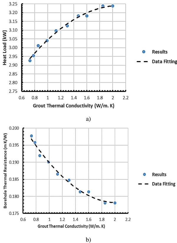
Fig. 3. a) Heat load variation with grout thermal conductivity at soil thermal conductivity of (2.42) W/m.K; b) Borehole thermal resistance variation with grout thermal conductivity at soil thermal conductivity of (2.42) W/m.K.
