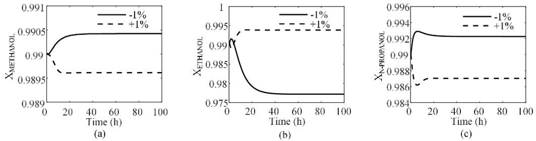
Fig. 5. Open-loop responses in face of  $\pm 1\%$  step change in feed flow rate: (a)  $x_{\text{methanol}}$  in the top of the PRE, (b)  $x_{\text{ethanol}}$  in the top of the SIDE, (c)  $x_{\text{n-propanol}}$  in the bottom of the STRI.
