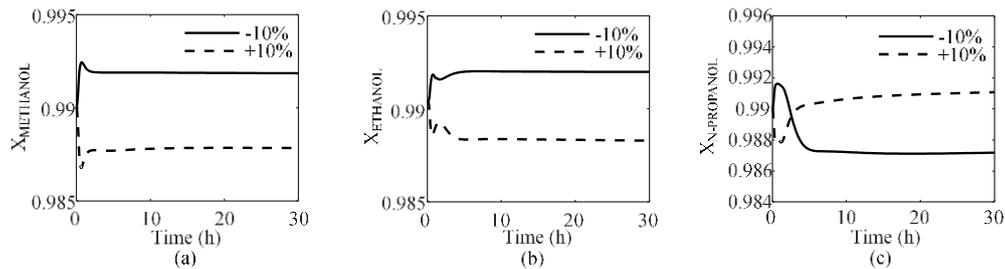
Fig. 7. Closed-loop responses in face of  $\pm 10\%$  step change in feed flow rate: (a)  $x_{\text{methanol}}$  in the top of the PRE, (b)  $x_{\text{ethanol}}$  in the top of the SIDE, (c)  $x_{\text{n-propanol}}$  in the bottom of the STRI.
