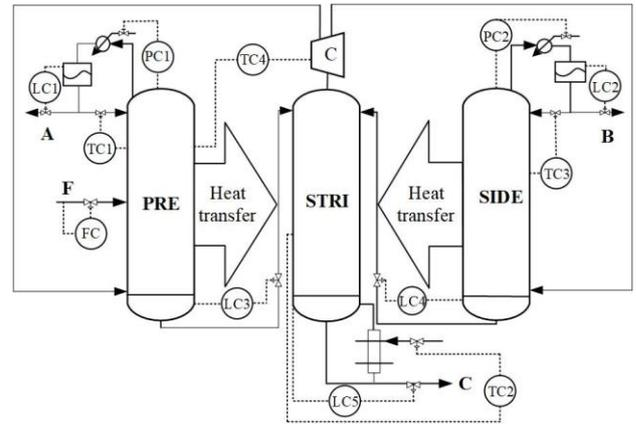
Fig. 3. Temperature control scheme of IHI-TDWC.
