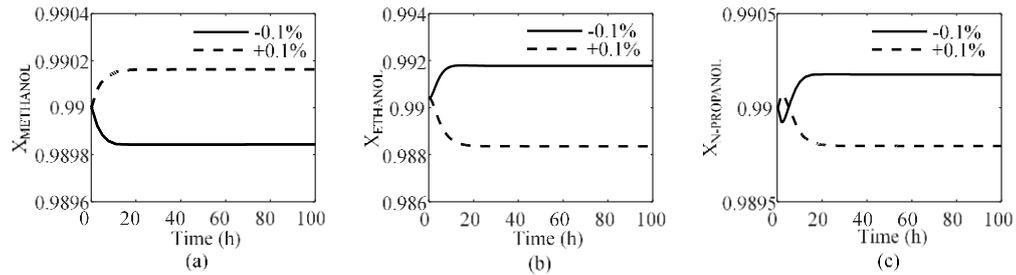
Fig. 6. Open-loop responses in face of  $\pm 0.1\%$  step change in feed composition of methanol: (a)  $x_{\text{methanol}}$  in the top of the PRE, (b)  $x_{\text{ethanol}}$  in the top of the SIDE, (c)  $x_{\text{n-propanol}}$  in the bottom of the STRI.
