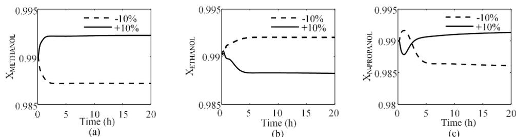
Fig. 8. Closed-loop responses in face of  $\pm 10\%$  step change in feed composition of methanol: (a)  $x_{\text{methanol}}$  in the top of the PRE, (b)  $x_{\text{ethanol}}$  in the top of the SIDE, (c)  $x_{\text{n-propanol}}$  in the bottom of the STRI.
