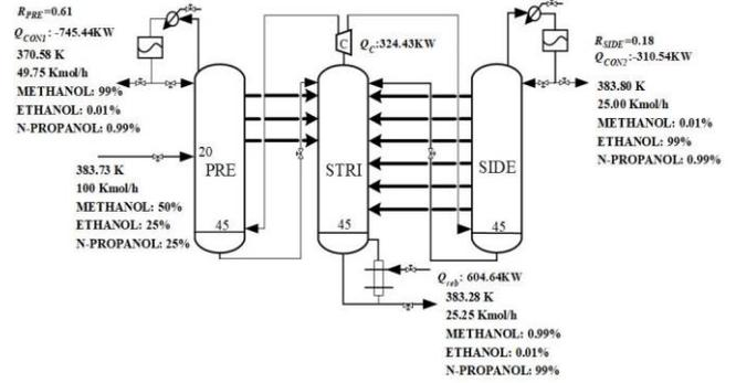
Fig. 2. Process design of IHI-TDWC.
