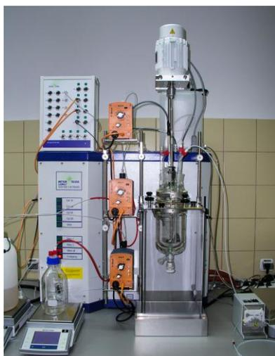
Fig. 1. Photo of experimental plant – continuous reaction crystallization of struvite (Mettler Toledo).
