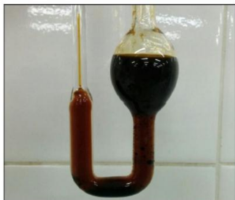
Fig. 5. Phase separation in the bio-oil, after 11 days storage at 40 °C.
