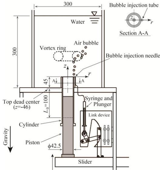
Fig. 2. Vortex ring launcher.
