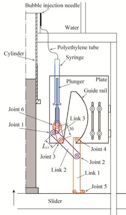
Fig. 5. Device to inject bubbles into water tank.
