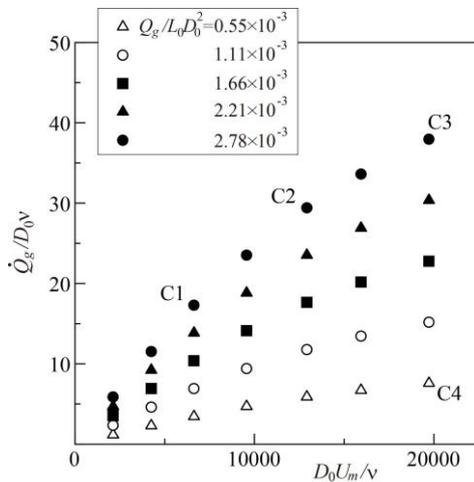
Fig. 7. Experimental condition for bubble injection.
