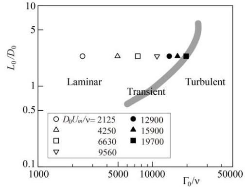
Fig. 4. Experimental condition for launch of vortex ring plotted on the identification map of Glezer (1988).
