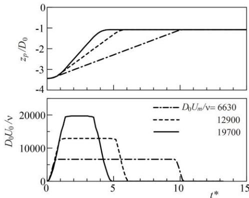
Fig. 3. Displacement and velocity profiles of piston.
