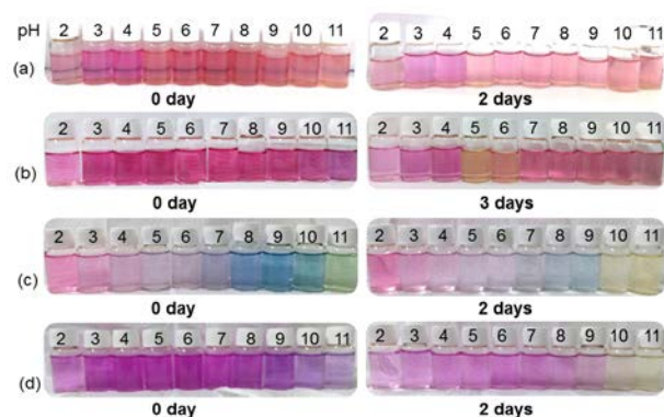
Fig. 1. Color disparities of encapsulated red biocolorant prepared from red spinach (a), beetroot (b), red cabbage (c), and dragon fruit (d), redissolved in buffered aqueous solution at pH 2 – 11 and after storage ( 20^{\circ}\text{C} , dark).
