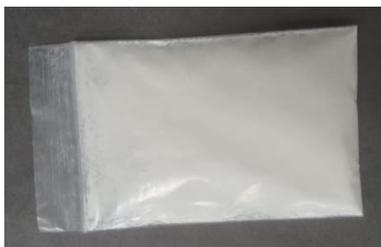
Fig. 1. Sample of n-MgO in powder form.
