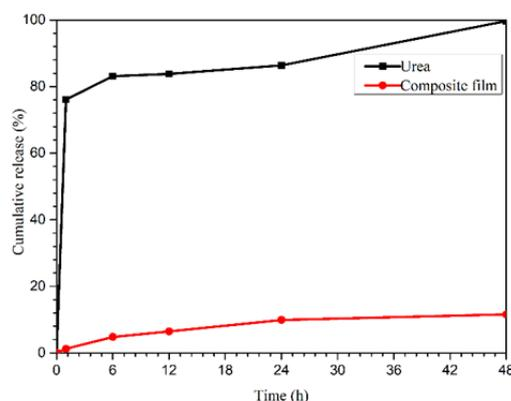
Fig. 4. Release behaviors of urea in water.
