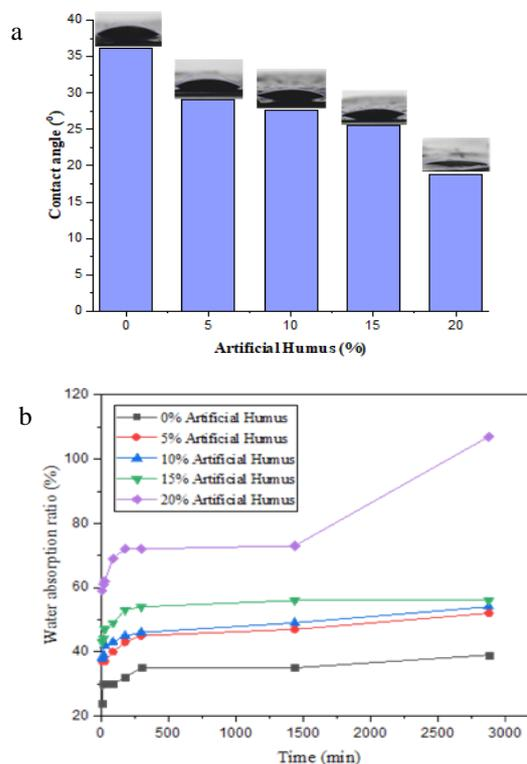
Fig. 2. Effects of different AH additions on the film: (a) contact angle and (b) water absorption.
