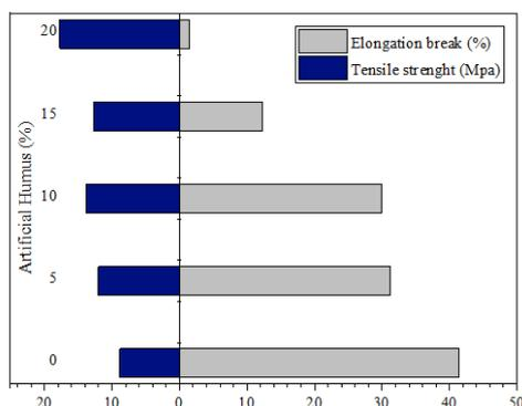
Fig. 1. Effect of different AH addition on the mechanical properties of the film.
