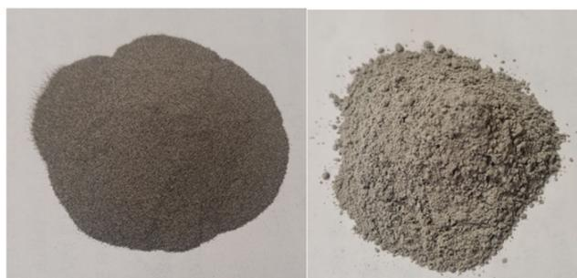
Fig. 1. Ground materials: BFS (left) and LS (right).
