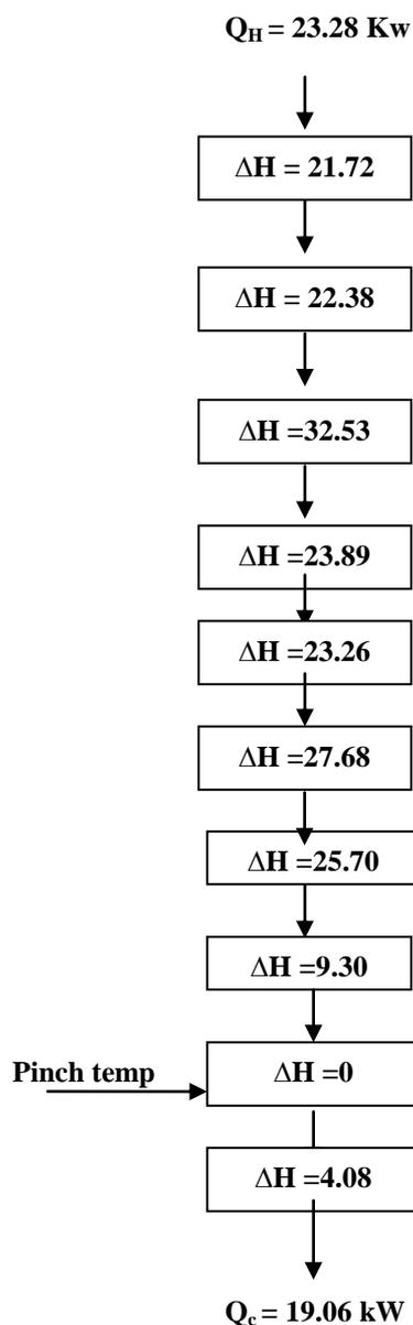
Fig. 2. A cascade diagram
