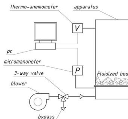
Fig. 1. Schematic diagram of the cold experimental unit
