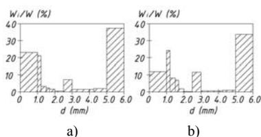
Fig. 8. Fractional composition of a bed material: a) after 40 minutes of start-up; b) after 90 minutes of start-up
