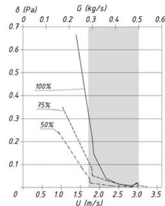
Fig. 7. Dimensionless amplitude of pressure fluctuations vs. primary air flow rate at 50%, 75% and 100% boiler workload of the nominal
