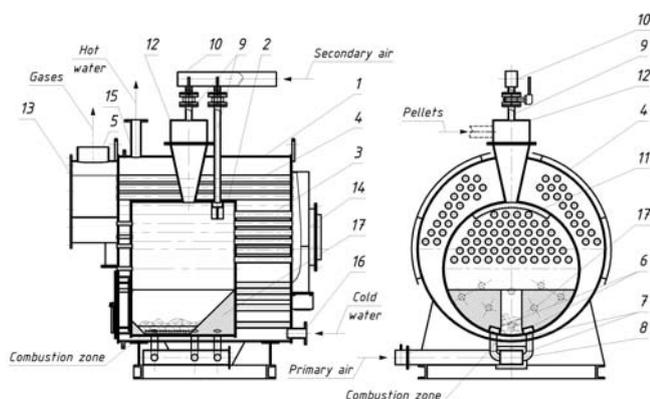
Fig. 2. Experimental boiler (hot model) diagram
