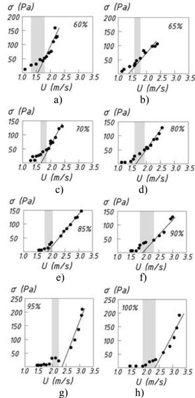
Fig. 5. The dependence of the standard deviation of differential pressure fluctuations vs. of air velocity for mixtures of: a) 60 and 40%, b) 65 and 35%, c) 70 and 30%, d) 80 and 20%, e) 85 and 15 % f) 90 and 10%, g) 95 and 5% pellets and particles of coal ash respectively, h) for a bed of straw pellets
