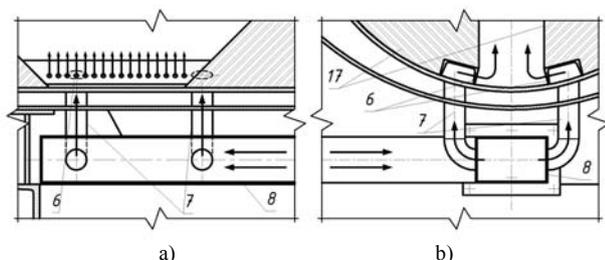
Fig. 3. Air distribution grill system and primary air supply diagram: a) longitudinal section; b) cross section
