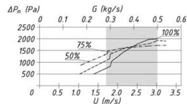
Fig. 6. Pressure drop in a burning bed vs. air flow rate
