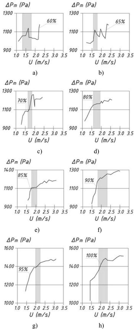
Fig. 4. Dependence of pressure drop in the bed vs. air velocity for mixtures of: a) 60 and 40%, b) 65 and 35%, c) 70 and 30%, d) 80 and 20%, e) 85 and 15 % f) 90 and 10%, g) 95 and 5% pellets and particles of coal ash respectively, h) for a bed of straw pellets
