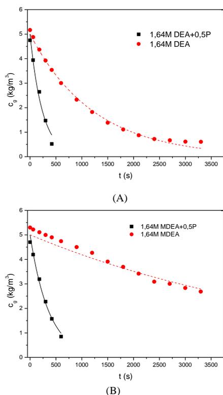
Fig. 4. Kinetics of CO<sub>2</sub> absorption in the membrane contactor for secondary (A) and tertiary (B) amines with and without presence of piperazine
