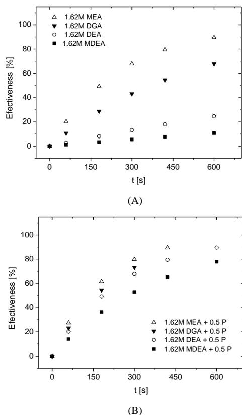
Fig. 3. Effectiveness of CO<sub>2</sub> absorption for amine solutions (A) and amine solutions with addition of piperazine (B) during the process of membrane absorption
