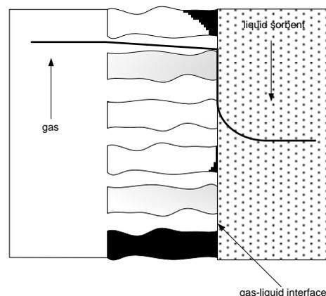
Fig. 1. Concentration profile in a membrane contactor.
