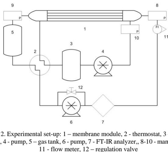
Fig. 2. Experimental set-up: 1 – membrane module, 2 - thermostat, 3 – liquid tank, 4 - pump, 5 – gas tank, 6 - pump, 7 - FT-IR analyzer., 8-10 - manometer, 11 - flow meter, 12 – regulation valve
