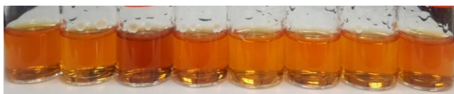
Fig. 1. Color changes observed upon the addition of various cations to the solutions of sensor L1 ( 1.5 \times 10^{-3} M) in ACN/H 2 O (10:1, v:v, pH 7.0) solutions. Left to right : free L1, Co 2+ , Cu 2+ , Cr 3+ , Mn 2+ , Zn 2+ , Ni 2+ and Fe 2+ .
